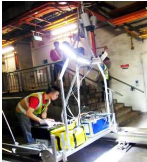
Fig 1: Kinematic High Resolution Imaging of track slab
