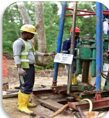
Undisturbed soil sampling : Mazier Sample
