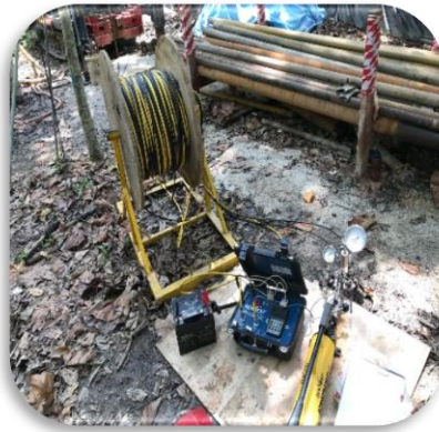
From left to right: Packer Test, Dilatometer Test readout, Lowering of Dilatometer probe into borehole
