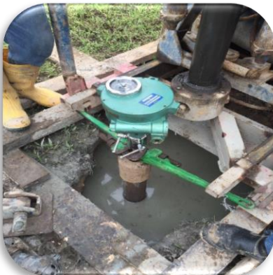
From left to right: Vane Shear Test, Downhole Seismic survey, PS Suspension Logging
